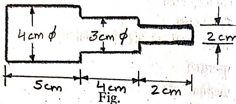
6. Estimate the cost of metal sheet for preparing a funnel as shown in fig. Assume the wastage of metal as 10% and cost of the sheet as @ ₹ 20/m<sup>2</sup>. 10
